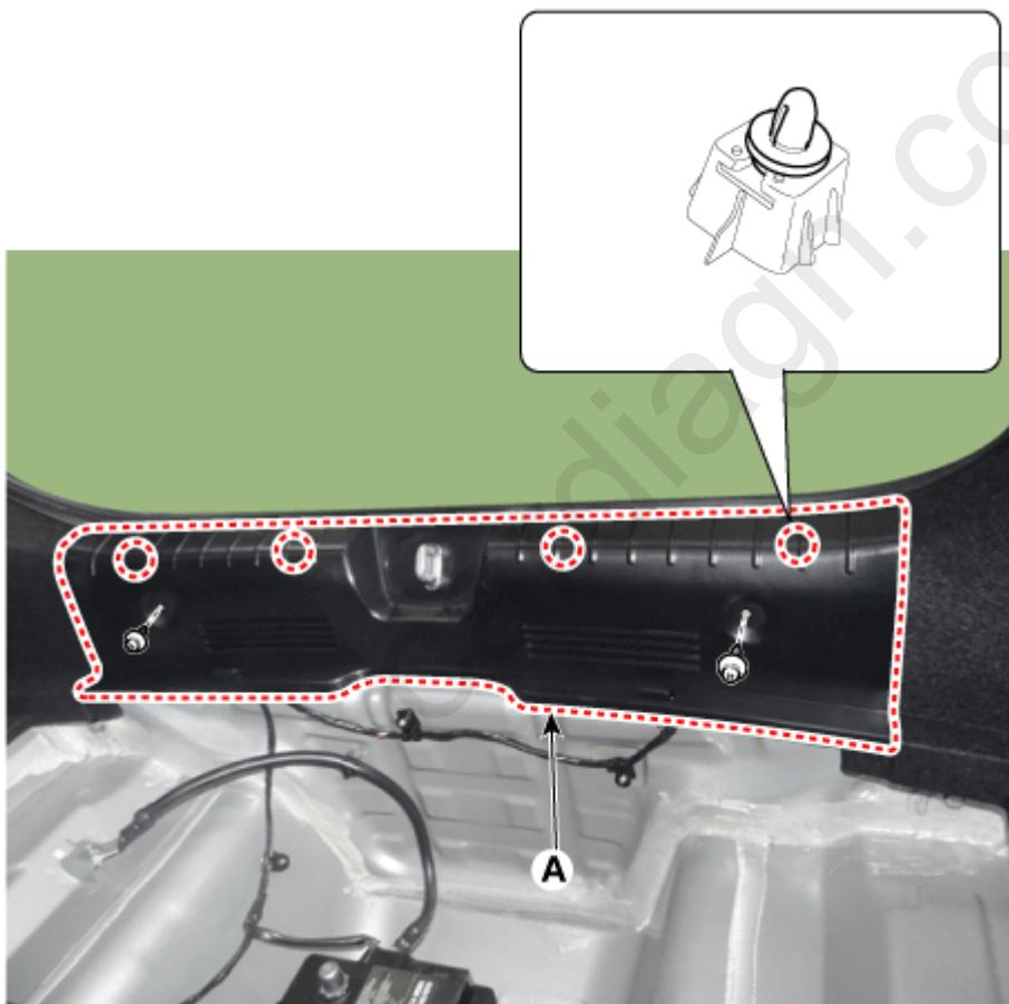
5. Separate the luggage side trim (A) after loosening the mounting screws.
